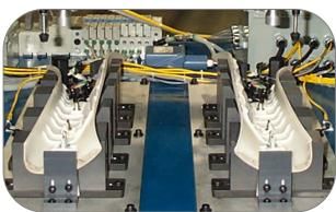
Ford A Pillar And Speaker Clip Installation, Hot Air Cold Stake
